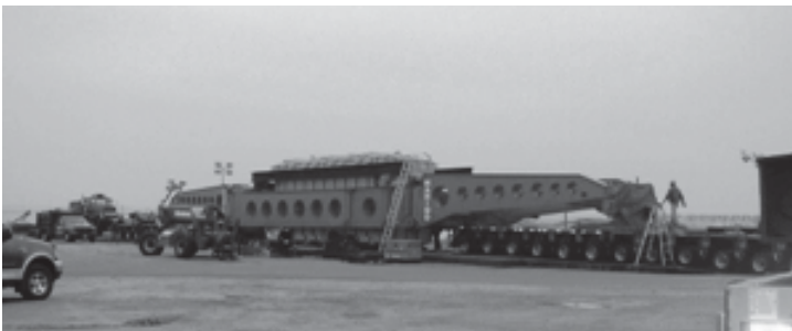
At Marino's job in Seabrook they are moving a 300-ton transformer on a 240-ft trailer to Londonderry. The move will take at least 4 nights.
